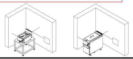
Relocation; The device, assembled by the Authorized Service, may not be RELOCATED by any person other than the authorized service. **ELECTRICITY SUPPLY CABLE MAY NOT BE EXTENDED, REPLACED.**
